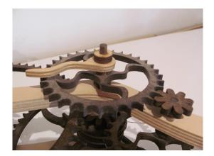
5) Push the second hand onto the escape wheel arbor protruding through top of front frame (do not glue). Make sure that the second hand does not contact the frame.
