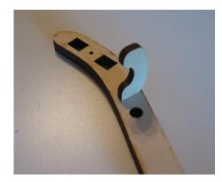
6) Apply a small amount of glue around the rim of each of the nine holes on the interior sides (shown face up in the photo below) of both frame pieces (5 in front frame piece, 4 in rear frame piece). Snap a nylon shoulder washer into each of these holes (it might be necessary to tap into place with a hammer).
