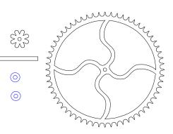
Mount the 60-tooth gear and the 8-tooth gear on arbor in
