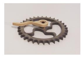
3) Push or twist a set washer onto the great wheel arbor until it is about 1/8" from the front of the frame. Slide the hour pipe (installed in 32-tooth gear) onto the great wheel arbor. The 32-tooth gear should mate with the 8-tooth gear.
