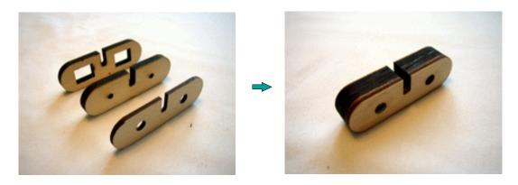
2) If desired, sand the perimeter of the completed upper hanger unit.
