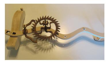
4) Insert the mid arbor into the next bushing, with the 8-tooth gear down. Be sure there is spacer washer at both ends of the arbor. The 60-tooth gear should mate with the 8-tooth gear on the escape wheel arbor.
