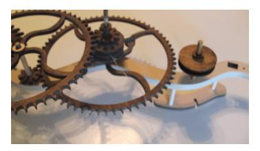
7) Carefully attach the front frame unit. Note that the escape wheel arbor and great wheel arbors extends through the front frame. Line the arbors up with the bushings as the frame front is applied. NOTE: the strut forks should slip into the rear frame holes. Some sanding may be necessary if the parts were slightly misaligned or there was glue residue on the strut forks or in the holes.
