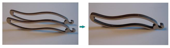
2) Separate the weight shell cover plate (#23) from the weight shell back (#24).
