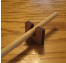
Apply graphite to the contact areas of the arbors by coloring that section of the arbor with a pencil.
