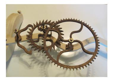
5) Insert the great wheel arbor into the next available bushing, with the 64-tooth gear down. Be sure there is a spacer washer adjacent to the 64-tooth gear. The 64-tooth gear should mate with the 8-tooth gear on the mid arbor. (Note: the 10 tooth gear on the great wheel arbor does NOT mesh with the 60-tooth gear nearby.)
