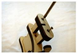
11) Attach (but do not glue) the crutch to the escape lever arbor protruding through the rear of the clock frame. Orient the crutch so that it is approximately perpendicular to the escape lever (the exact position of the crutch will be adjusted after the clock is mounted on the wall). The crutch should fit firmly on the arbor so it cannot slip on the arbor.
