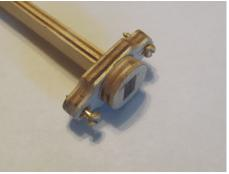
If the fit is not snug, use a piece of tape to hold the bracket in this position. Thread the pendulum between the crutch forks, and up toward the pendulum support plate. Place the screw tips onto the two small holes in the pendulum support plate. NOTE: <u>The screw tips simply rest in the pendulum support plate holes</u>; these screws do not get driven into the pendulum support plate.
