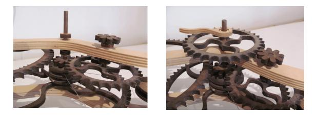
4) Push or twist a set washer onto the great wheel arbor until it is about 1/16" from the hour pipe. There should be just enough clearance to hold the hour gear in position while still allowing it to rotate. Next, twist the minute hand onto the great wheel arbor. As with the hour hand, the fit should allow the minute hand to be repositioned on the arbor.
