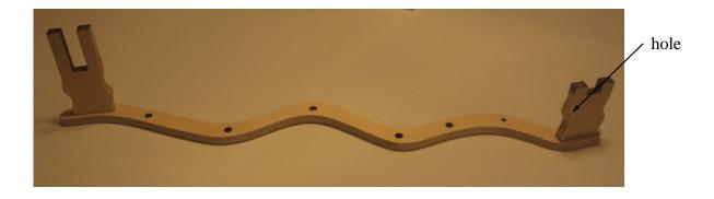
4) Glue the lower support bracket unit into holes in rear frame piece with the slot oriented as shown below.
