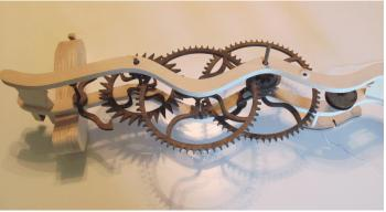
8) Drive a #4 x 1" screw through each of the two the predrilled hole in the back side of the rear frame piece. The screw holds the rear frame piece tight to the upper and lower struts.
