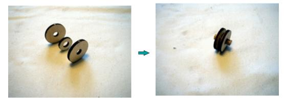
2) Glue one of the pulley faces (#52) onto one of the pulley frames (#6). Repeat for the other pulley face and pulley frame, except glue the pulley face to the opposite face of the frame piece (look ahead to step 4).
