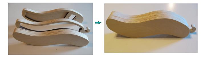
7) Perform any final sanding on the weight shell and finish as desired.
