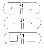
1) Glue together the three upper hanger bracket pieces (#54, #17, #15) with the pieces aligned as shown below.
