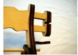
10) Drive two #4 x 1" screws through the predrilled holes in the back side of the hanger bracket into the upper strut.
