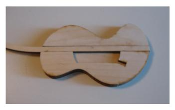
8) Remove the shaft. Glue the pendulum clamp (#12) into the slot in the back of the pendulum bob with the cutout section over the slot that runs down the middle of the bob. Apply glue only to the portion of the clamp that fits into the slot in the bob (the rest of the length must be free to flex).
