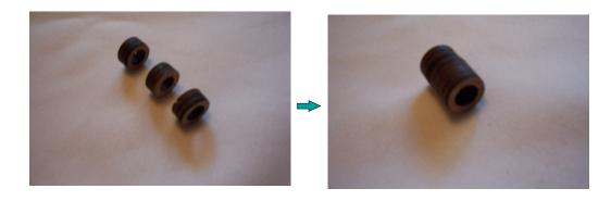
2) After hour pipe glue is completely cured, use a hammer to gently tap the minute pipe into the 32 tooth gear:
