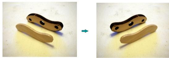
3) Sand the perimeter of the two pulley side units.
