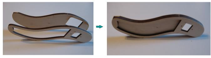
4) Glue together the weight shell front (#18) and the two weight shell middle pieces (#27) oriented as shown below with the perimeter edges aligned.
