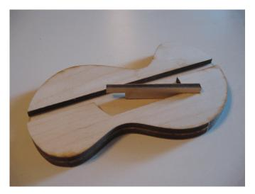
9) Sand the perimeter of the pendulum bob and apply finish as desired.
