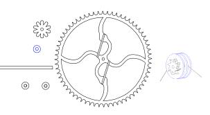
note: hour gear, set washers, and minute hand will be installed on this arbor after clock is assembled.
